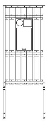
Please note: Before concreting, ensure the anchor posts are attached to the frame – do not attempt to concrete the anchor posts by themselves. Try to avoid concreting the letterbox frame into the ground, it is preferable that only the anchor posts go into the concrete.
